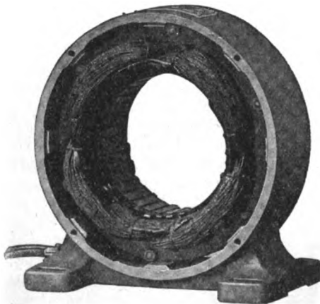
FRAME WITH BRACKETS AND ROTOR REMOVED, SHOWING PRIMARY CORE AND WINDINGS
